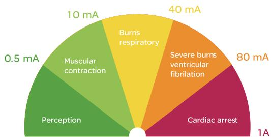
By measuring the intensity difference between live and neutral conductors, RCDs actually detect the current flowing through the human body. If this current reaches the 30 mA limit, the RCD trips within a few milliseconds, so preventing injury or worse.
